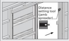
e) Without moving the activator, open the door and securely tighten all four activator grub screws.
