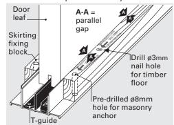
Concrete floor: Ø8 x 90mm masonry anchor Timber floor: Ø3.15 x 75mm nail (not supplied)
