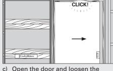
activator grub screws. The cassette is now charged. 2.d) Position the distance setting tool (jamb spreader) against the centre of the closing jamb and gently close the door onto it.
