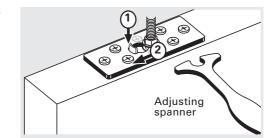
19. Once the plunger is fully depressed, slide the spanner sideways towards the plunger pin.
